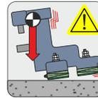
Anchoring top-heavy machines to the floor Bolt-on Jacmount Adjustable Levellers may not be used on top-heavy machines!
